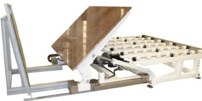
Automatic loader of the slab from L-frame to conveyor belt
